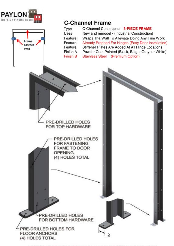
ROUGH OPENING WIDTH = FINISHED OPENING WIDTH + 1.25" ROUGH OPENING HEIGHT = FINISHED OPENING HEIGHT + .625"
