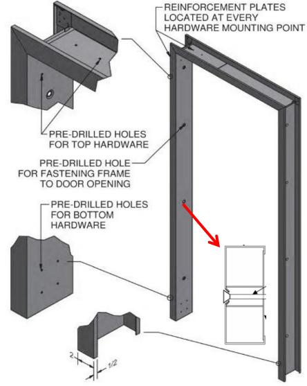
ROUGH OPENING WIDTH = FINISHED OPENING WIDTH + 4 3/8"
